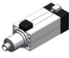
MT1120 - H6162H0122 Kw 13,50 S6 - ER40 collet - 18.000rpm - 380V - right rotation
