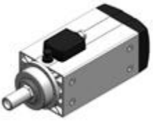
MT1120 - Y6164Y0020 Kw 8,10-S1/9,50-S6 - special connection - 6.000rpm - rated voltage 380V - right rotation
